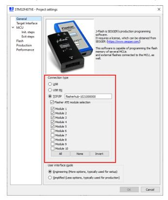
When selecting "File > Download config & data file to Flasher" from the J-Flash menu, the configuration and data file of the current J-Flash project will be downloaded to the selected Flasher Compact modules.
